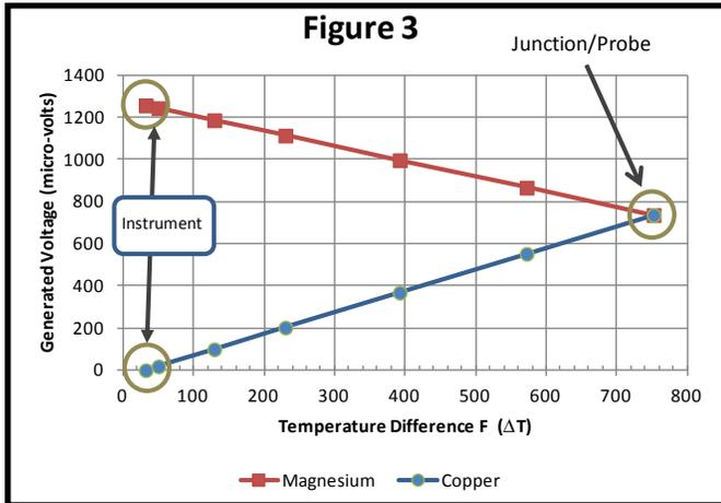
uncompensated instrument), or a local cockpit temperature measurement is made internally (referred to as a compensated instrument). One quick way to determine if you have a compensated gage or not is to look at the temperature reading when it is cold outside (say 30° F). If it reads close to 30° F then most likely you have a compensated gage. If it reads 70° F, chances are it is uncompensated. Always refer to your particular
